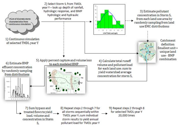
Figure 4. SBPAT Monte Carlo Method Components
