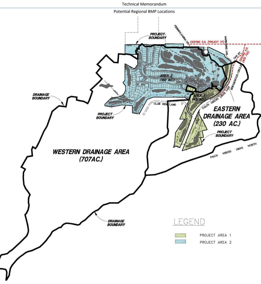
Figure 4: Chandler Quarry Project Drainage Area Map (Hunsaker and Associates. Water Quality Mitigation Plan. June 16, 2010).
