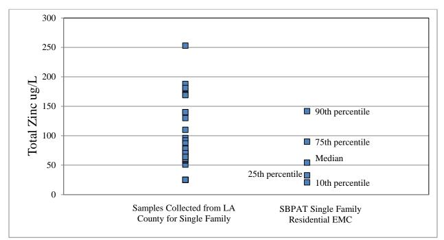
Figure E-7: Comparison of SFR monitoring data and SBPAT modeling data for total zinc
