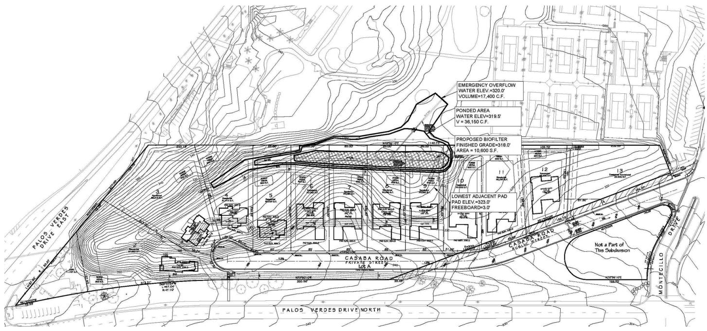
Figure 3-6: Casaba Estates (formerly Butcher Ranch) Post-Development Design Conditions (Bolton Engineering Corp. Hydrology and Hydraulic Calculations. September 13, 2010).
